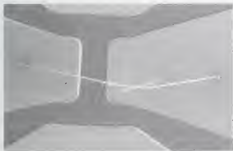
Figure 1. SEM image of carbon nanotube test device for electrical measurements. The nanotube extends across a 2 \mu\text{m} gap.
